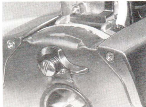
Figure 4. Cover Assembly Removal
