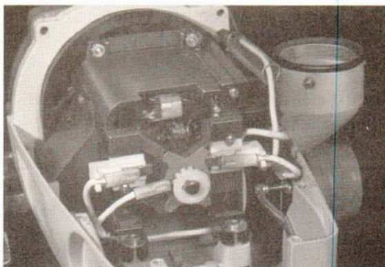
Figure 12. Motor Unit Assembly Removal (Top)
