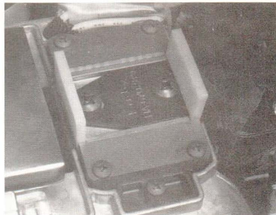
Figure 21. Handle Pivot Spring Assembly Shim Tool Use
