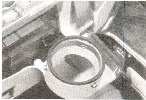
Figure 18. Exhaust Horn Gasket Removal
