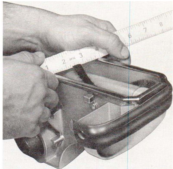
Figure 2-2. Checking nozzle brush protrusion
