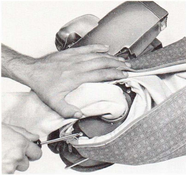
Figure 4-4. Filler tube, adapter collar, and mounting screws
