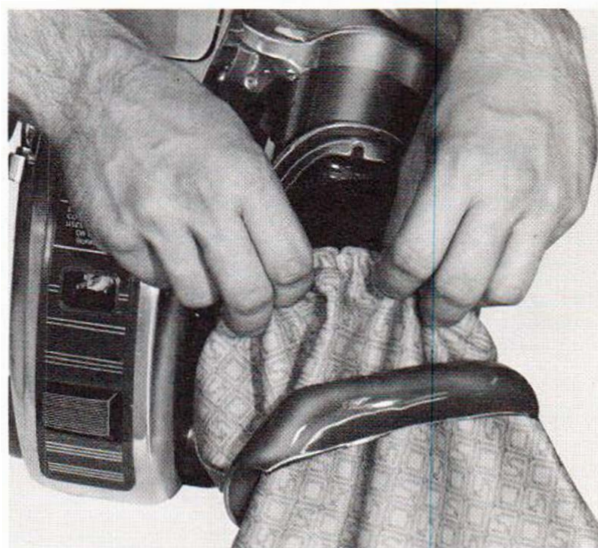
Figure 4-3. Installing bag on Sani-Em-Tor body
